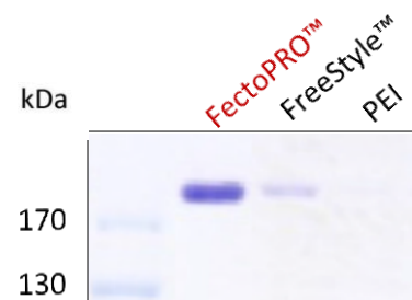
Fig 1: FectoPRO™ gives superior protein production yields in suspension CHO cells. FreeStyle™ CHO cells were seeded at 1 x 10 6 cells/ml in 30 ml of FreeStyle™ CHO Expression Medium and transfected with FectoPRO™ (0.8 µg DNA/ml), FreeStyle™ MAX Reagent (1.25 µg DNA/ml) or PEI (1 µg DNA/ml) following recommended protocols for the respective reagents.
